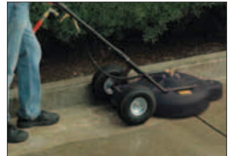
The Cyclone attaches to a hot- or cold-water pressure washer and 'mows' grime fast
